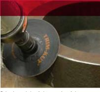
Deburring and chamfering a section of pipe after cutting.
