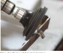
Edge chamfering a fabricated stainless component.
